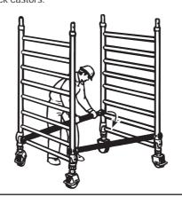
6 Clip first diagonal braces (blue) as shown. Adjust legs to ensure tower shown. Adjust legs to ensure tower is vertical and square and that horizontal braces are level, using a spirit level.
