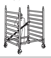
Position fixed deck on fourth rung of frames as shown Position and a live frames as shown. Position second lift of frames and engage interlock clips.
