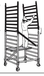
Clip on third diagonal braces (blue) as shown. Ensure that separate frames are always braced together. Locate Trapdoor Deck
