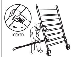
Clip other end of horizontal brace onto other frame. Clip second horizontal brace onto other side of frames. Ensure claws are locked outwards never inwards. Lock castors.
