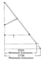
SP15 Stabiliser Weight: 12.70Kg Code: 319513
